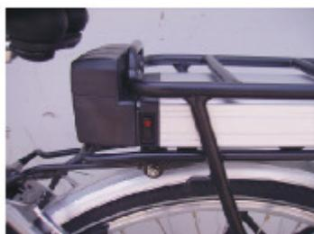
fig.2 battery main switch
